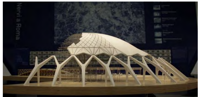
Fig. 12. The 1:25 scale model of the Palazzetto dello Sport, 2010 (Photo Sergio Poretti, MAXXI Pier Luigi Nervi Exhibition, Roma).
