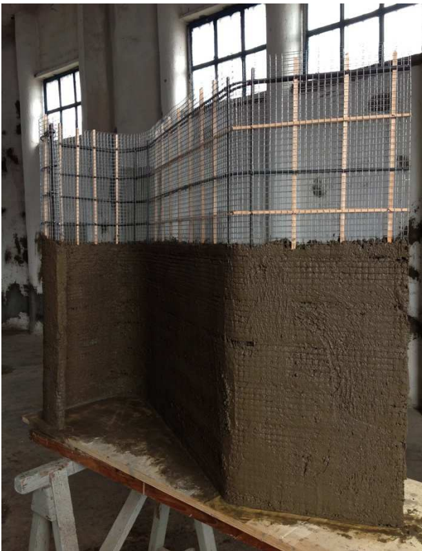
Figure 5. Full size model of a portion of the Magliana Warehouse's curly wall, 2013
